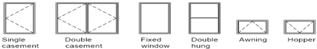
Figure 1.1 Examples of window symbols in elevation view
